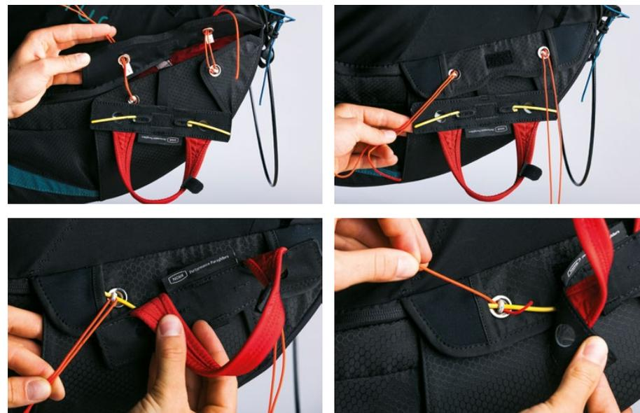
7 Once the rescue container is closed, correct deployment of the parachute must be tested. Slowly and carefully remove the piece of paraglider line from the closing loops and pull the red deployment handle. If the instructions were followed closely and everything was fitted perfectly, then the yellow rods will release and the parachute can be pulled out of the rescue container with very little effort. The required force must not exceed seven (7) daN.
