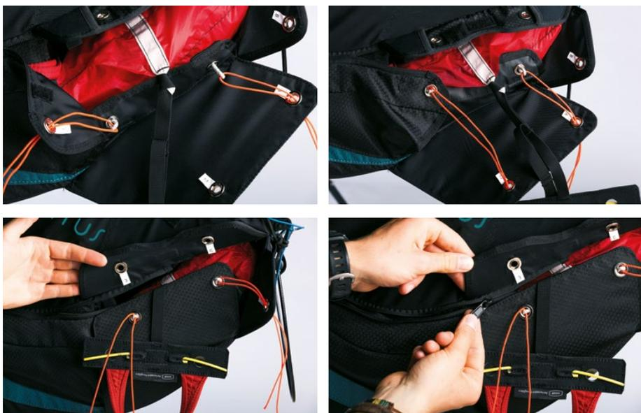
If the parachute is deployed, the zip on the right hand side will open. The zip must now be closed again. The important thing is to first guide the zip to the start of the rescue container and then all the way to the zip gate at the neck area, to ensure that the entire zip is fully closed.
