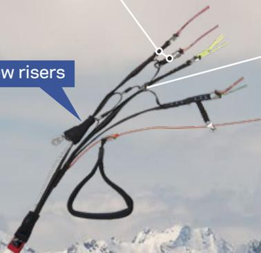
Ronstan ball bearing pulleys on the speed-system.
