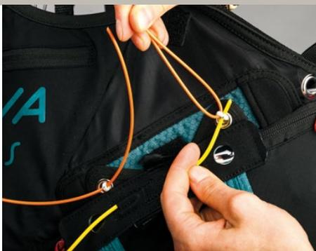
**3.2:** The pieces of paraglider line or small rods are now threaded through the eyelets of the closing flap underneath. By pulling on the line or the small rods the flap is closed and the white loops have been pulled through to the outside. Now the yellow closing pins of the deployment handle can be passed through the white loops one after the other.
