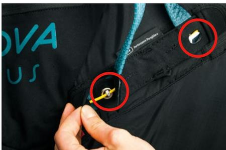
After removing the lines or the small rods, the yellow closing pins and the black tabs of the rescue handle must be stored in the elastic side pockets of the rescue container. Using the two round windows it is possible to check whether the yellow rods are located properly.
