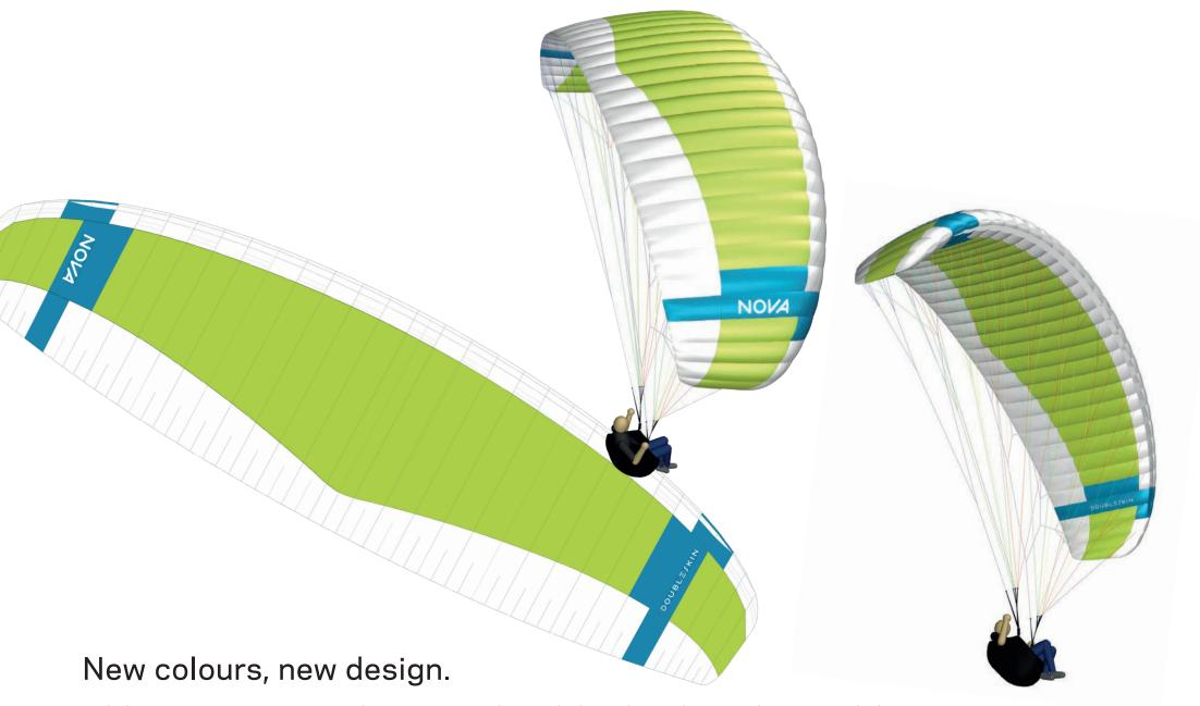
With the DOUBLESKIN, NOVA is introducing a new wing design. The basic design element is the "sweep", which emphasises the optical aspect ratio of the paraglider. On each wingtip there is also a "banderole" that will vary slightly in appearance from model to model, making room for manufacturer and product names. In the case of the cloth, new, vibrant tones enrich the colour palette previously used by NOVA.
