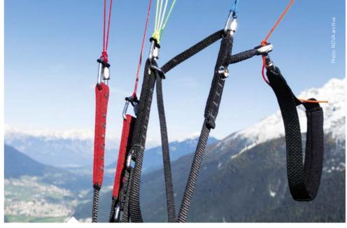
In accelerated flight, many pilots correct pitch and roll movements via the C-area. But this causes a performance limiting crease in the profile. If the C-riser of the NOVA Speed Brake Riser (SBR) is pulled back and down, this results in the B-area also being pulled down up to 50% via a pulley – without the performance killer crease.
