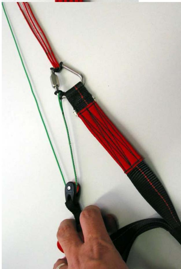
*By pulling the handle, the additional line gets under tension, pulling down the outer A line. The wingtips are collapsing.*
